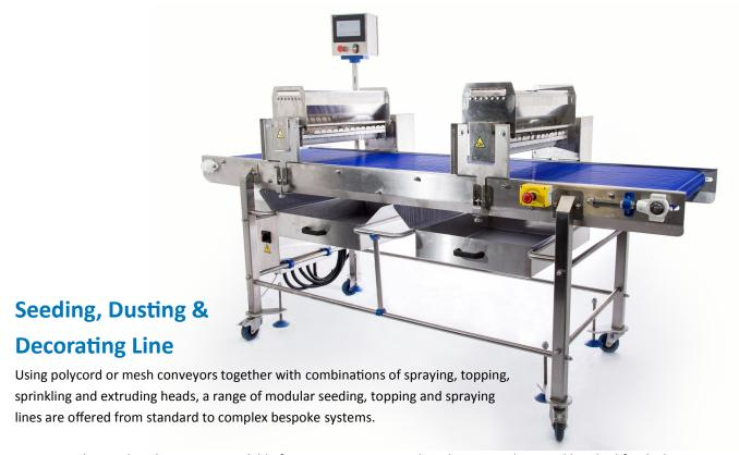
Starting with an indexed conveyor, available from 1.5 to 6 metres in length, on stainless steel brushed finish chassis, up to three heads can be mounted making this unit an ideal multipurpose system for dusting, seeding or sprinkling a wide variety of toppings onto a range of products.
